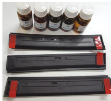
Figure 5: Surface energy measurement by inks.
