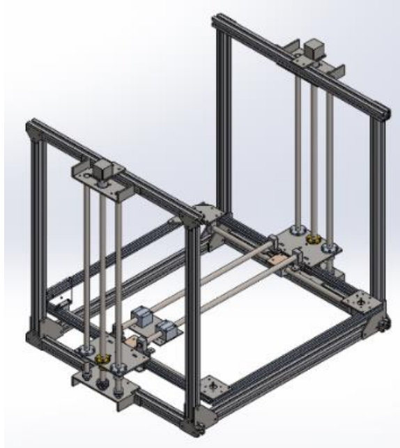
Figure 1. Design of Cartesian Magnetic Flux Mapper.
