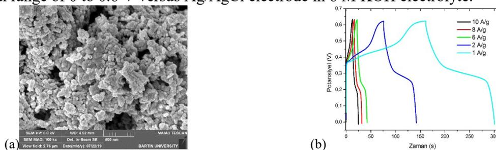
Figure 1. (a) SEM images and (b) charge-discharge curves of Ni Cu oxide electrodes
