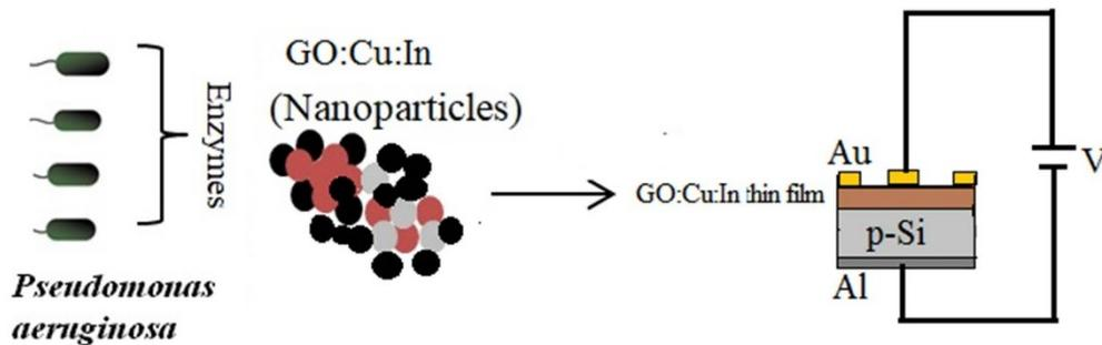
Fig. 1: Bacterial synthesis of GO: Cu: In nanoparticles and Au/ GO: Cu: In /p-Si/Al structure
