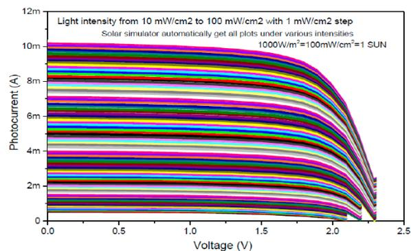
Fig.2. Solar Simulator system automatically measures current-voltage (I-V) under various light intensities
