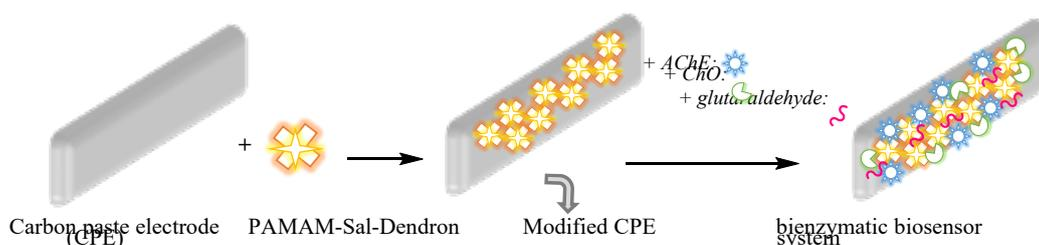
**Figure:** Bienzymatic biosensor design method
